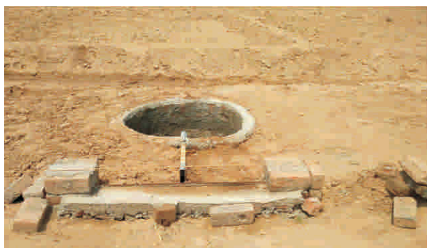
Fig. 11 a : Installation of Ramser sampler to measure the runoff and soil loss
