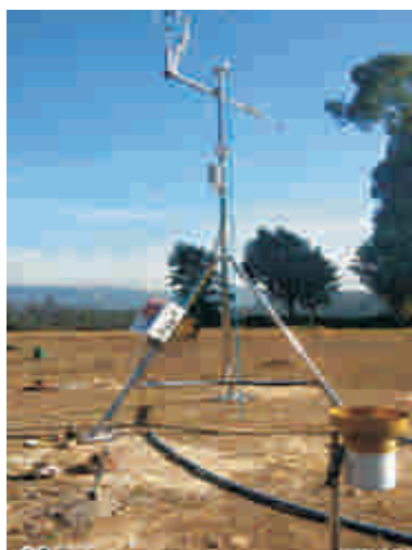
Plate 1 Eddy Covariance 1.3: Soil Carbon Dynamics and Erosion Productivity Studies
