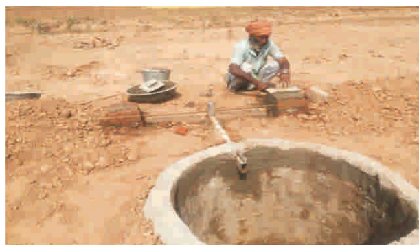
Fig. 11 a : Installation of Ramser sampler to measure the runoff and soil loss
