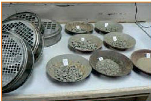
Fig. 7: Mechanical sieve analysis of filter materials for permeability and stability analysis of runoff filter
