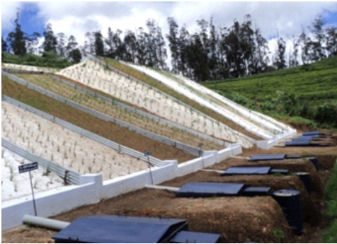
Plate 11. View of the grass establishment during final monitoring period in 60% slope
