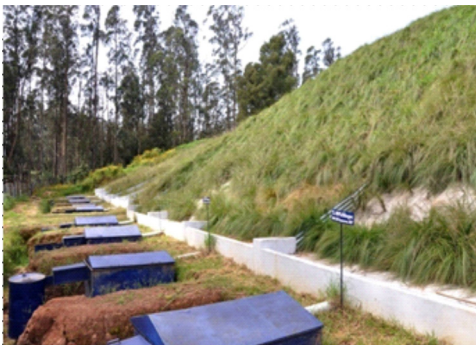
Plate 12. Photographs showing establishment of grass at various stages in 90% slope
