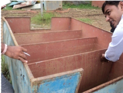
Plate 2. Runoff measuring devices installed at each plot (Multi-slot divisors)
