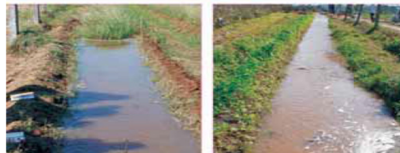
Runoff flow in vegetative waterways with varying grass filter coverage
