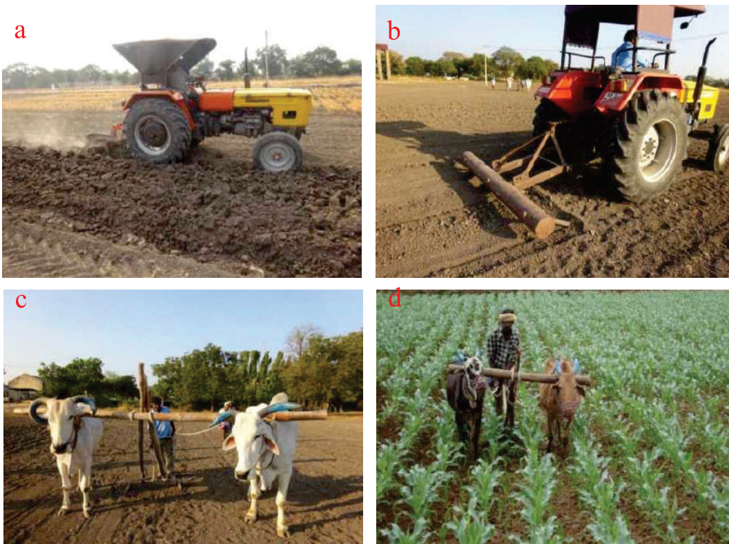
Plate 1: Various tillage practices being adopted in Vertisols of South India; mouldboard ploughing (a), tractor drawn blade harrowing (b), bullock drawn blade harrowing (c) and bullock drawn hoeing (d).
