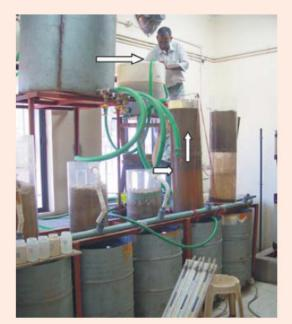
Laboratory set-up for testing efficiency of filter system comprising gravel, sand and agro-net in case of upward flow of runoff through filter system found suitable for area with slope < 4%.
